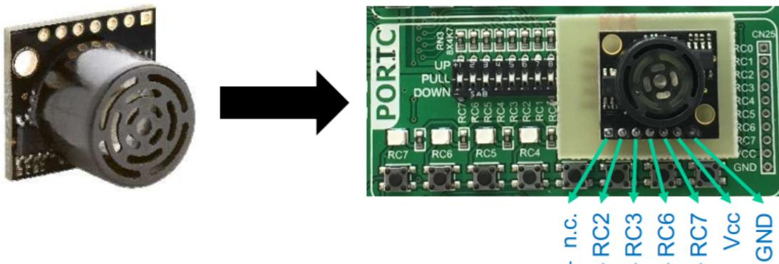
Pin 1 – Temperature Sensor Control: Not Connected
